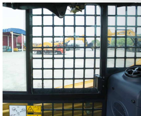
PROTECTIVE NET: It prevents personnel injuries caused by splashing or falling stones, etc.
