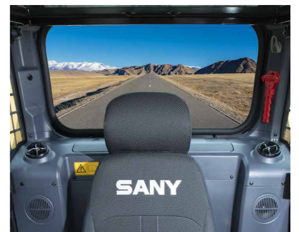
ESCAPE WINDOW: emergency exit.
