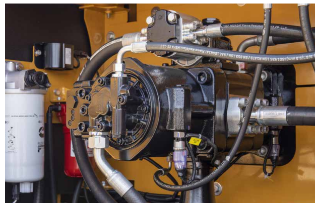
Main valve model: KMX15RB Rated flow: 300 L/min Rated pressure: 37.7 MPa
